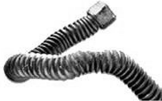
To our knowledge, these brass connectors have not been manufactured for over 20 years, but many are still in use. Not all uncoated brass connectors have this flaw, but all should be inspected by a professional and replaced with stainless steel connectors. Gas appliances in your home that should be checked include:
